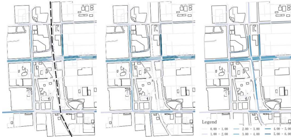
Fig. 2. NO x distribution from the COPERT model in the three design scenarios: baseline (left), scenario 1 (middle) and scenario 2 (right)
